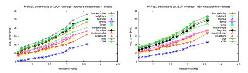
only the +12VDC EPS connector power is shown left observation: the two alternative measurement techniques coincide qualitatively and quantitatively for a wide range of frequencies small difference as the 24 PIN 5V connector also supplies the CPU (and other mainboard devices)
