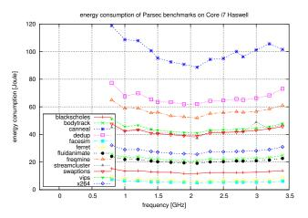
smallest energy consumption between 2 GHz and 2.5 GHz
