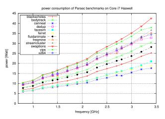
large variation of the power consumption for different benchmarks Benchmarks with a **sequential workload** typically lead to smaller power values
