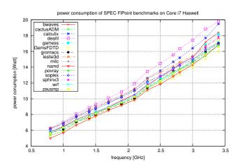
different applications lead to different power consumption slightly larger power consumption as for the integer benchmarks
